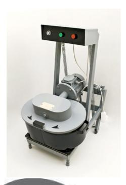
The laboratory mixer is designed for the preparation concrete mixtures to production of concrete samples. The mixer allows for good mixing into the volume of the 13l mixture.
