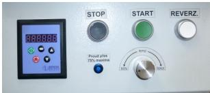
Blades of mixer HMB 35f rotates in the unloaded conditions with speed 20 to 100 RPM – this speed is adjustable by knob on the control panel. The stirred mixture is discharged by opening segment at the bottom of the vessel. To facilitate handling of the mixer are mounted on the frame casters, and on the frame handle.
