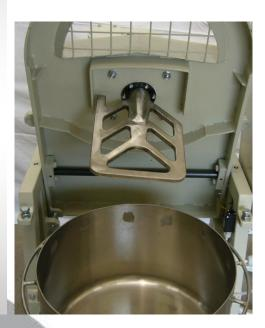
The mixer has separate drive for blade and for the mixing vessel. The blade is positioned eccentrically with respect to the container, here is the possibility of adjusting the technological gap between the blades and the bottom and wall of the container in the range of 2-20 mm. Control electronics panel is located on the side stand. It contains start and stop individual drives, central stop and main switch.
