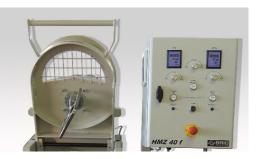
Mixer of refractories is designed for preparation of concrete mixtures and mortars to 26l in volume / according to consistency / for laboratories in the field of building materials.
