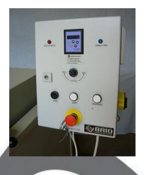
Cyclos type LMB-C1F is accompanied by a frequency converter for stepless speed control in the range of 20 to 60 rpm. Electric panel with PLC is placed firmly on the frame of the mixer.
