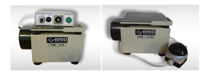
Vibrating table is designed for compacting concrete mixes in the test moulds. Thus made concrete sections are intended for further laboratory tests.
