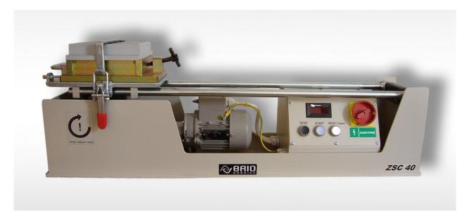
The equipment is intended for compacting the cement paste in the steel moulds and for the needs of other laboratory tests of cement.
