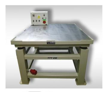
Low-frequency vibrational device is designed for compacting concrete mixture in the test labs. Vibration is due to mechanical vibrator EVU 500. Vibrations are adjustable in five stages via eccentric elements.
