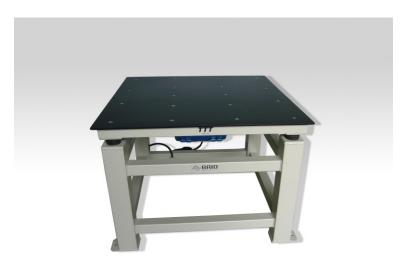
Low-frequency vibrational device is designed for compacting concrete mixture in the test labs. Vibration is due to mechanical vibrator EVU 500. Vibrations are adjustable in five stages via eccentric elements.
