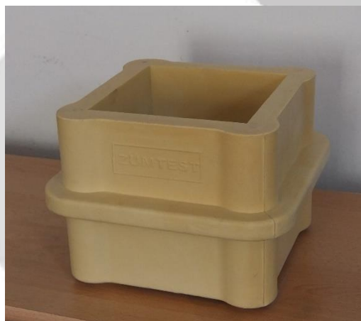
Full-plastic mould for cubes 150 mm /ZUM TEST/
