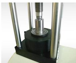
The press is designed for sample preparation (tablets) in X-ray fluorescence spectrometry, infrared spectrometry, for calorimetric measurements, etc.
