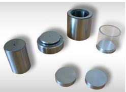
The press is designed for sample preparation (tablets) in X-ray fluorescence spectrometry, infrared spectrometry, for calorimetric measurements, etc.
