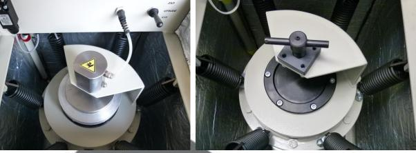
The device comes standard with a grinding bowl made of tool steel hardened 19436. May also be supplied from durable sintered material hardness GH13 1 100HV (87%  $\,$ WC, 13% Co).
