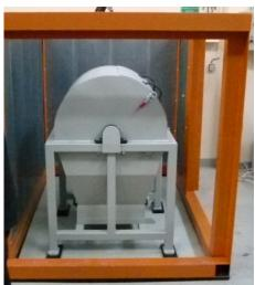
Ball mill is designed for discontinuous milling of the various materials (clinker, slag, limestone, etc.).
