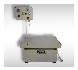
Vibrating table is designed for compacting concrete mixes in the test moulds. Thus made concrete sections are intended for further laboratory tests.
