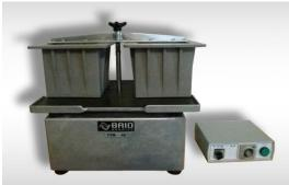
Vibrating table is designed for compacting concrete mixes in the test moulds. Thus made concrete sections are intended for further laboratory tests.
