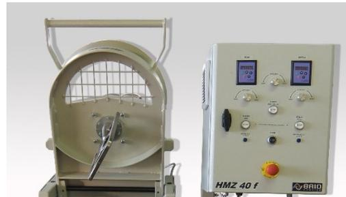
**Mixer of refractories is designed for preparation of concrete mixtures and mortars to 26l in volume / according to consistency / for laboratories in the field of building materials.**
